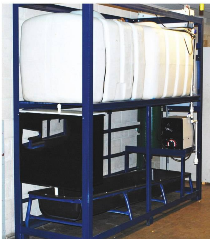
Compact EC system treating groundwater contamination at the Colorado Convention Center to meet discharge requirements.
